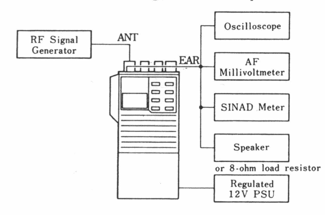
(7) Reduce the generator output so that only 2 segments are on, and confirm that the injection level is 5 dBµ or less.
