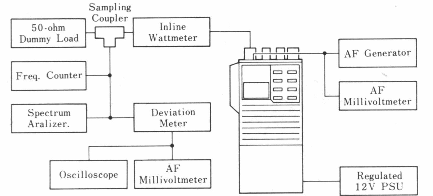
(145 or 146 MHz), adjust the AF generator for 25mV output at 1 kHz to the MIC jack.
